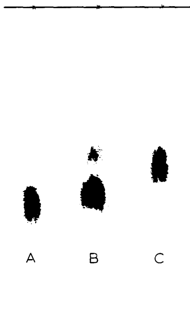
Fig. 4. Paper chromatography of the transferase products after separation from lactose. A, allolactose; B, sample from milk; C, 6- O - \beta -D-galactopyranosyl-D-galactose.
