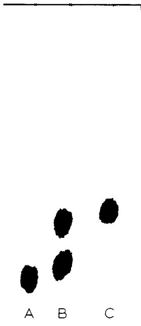
Fig. 1. The separation of glucose and galactose by paper chromatography. A, glucose; B, sample from milk; C, galactose.
